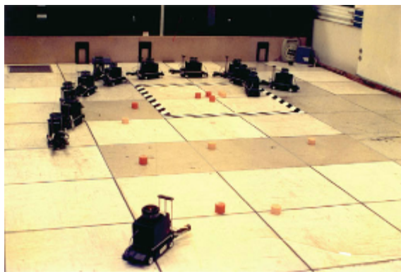
Figure 16.11 The Nerd Herd, together with the pucks that they can pick up with their grippers.
